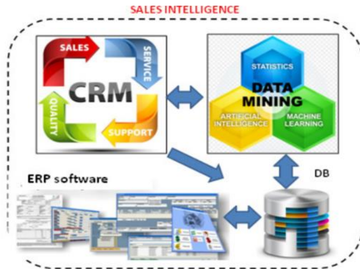
Fig. no. 10. Sales Intelligence platform: system architecture integrating a data mining engine (Massaro et al., 2018, p.41)
